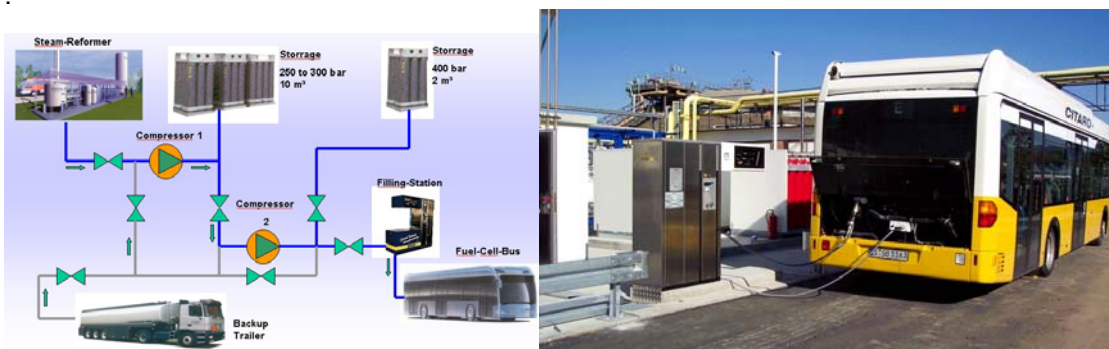
Figure 8 Stuttgart filling station layout
