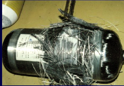
Hydraulic burst test
