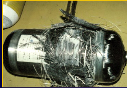
Hydraulic burst test
