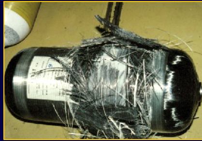
Hydraulic burst test
