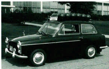
Figure 2 – K. Kordesch's prototype equipped with an AFC Union Carbide cell (6 kW) (1970)
