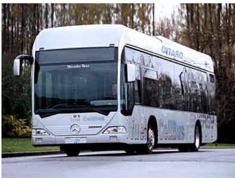
Figure 1 – The Citaro bus equipped with a Ballard fuel cell (CUTE project)
