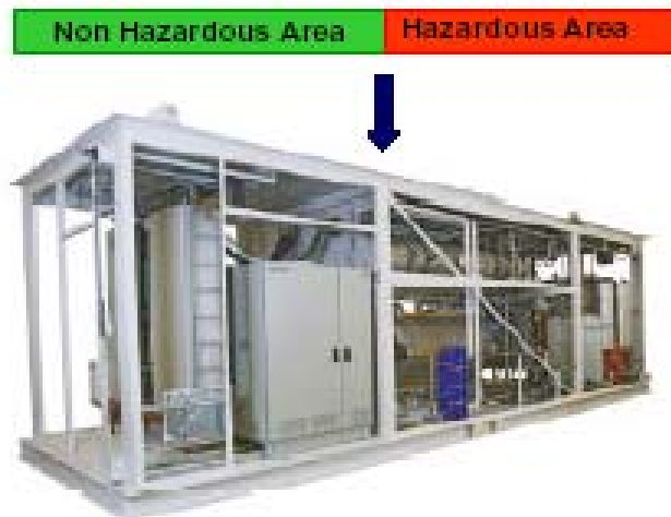
Figure 7: Containerized electrolyser without wall panels showing the electrolyser unit separated by a wall into hazardous and non-hazardous area.
