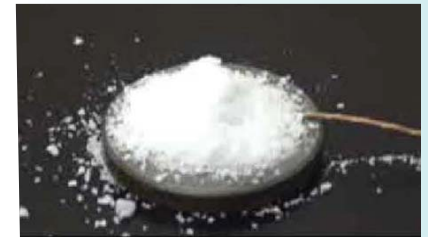
WATER DROP TEST - AMMONIA BORANE
