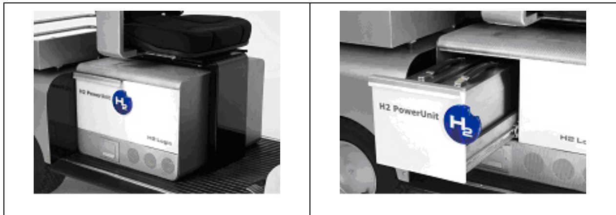
Figure 2: H2 PowerUnit installed on the H2 Truck with H2 Logic easy replace and fill system
