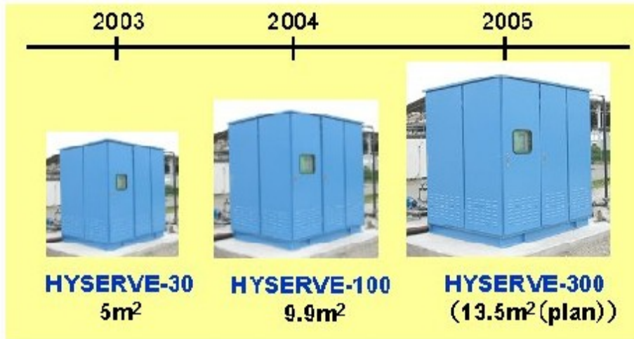
Fig. 5.3-2: Development of compact reformers 1
