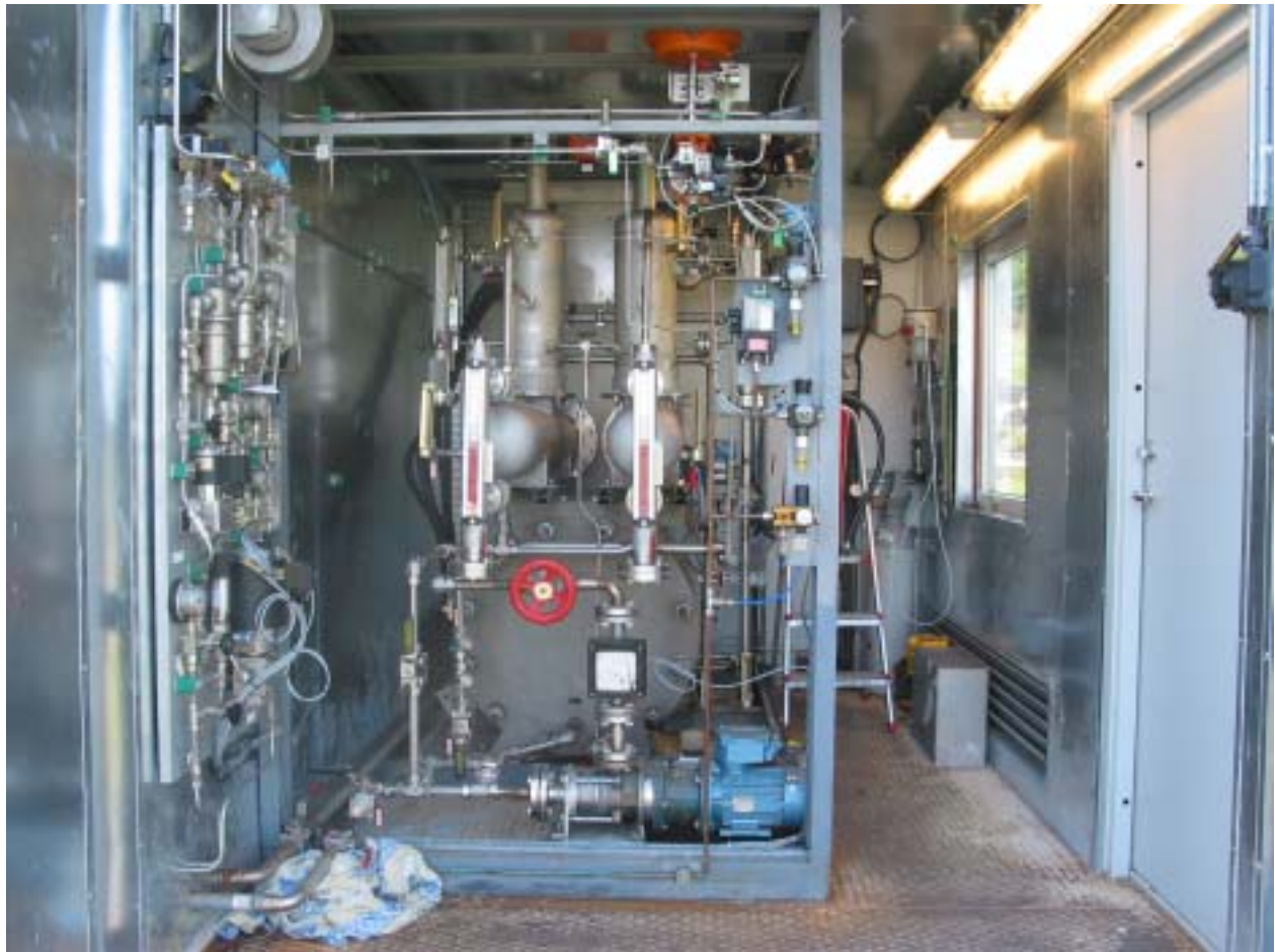
Figure 8: The 50 kW high-pressure alkaline electrolyser
